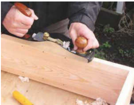
STEP 11. True up front and rear edges as necessary, taking care not to overrun with the plane and cause break-out
